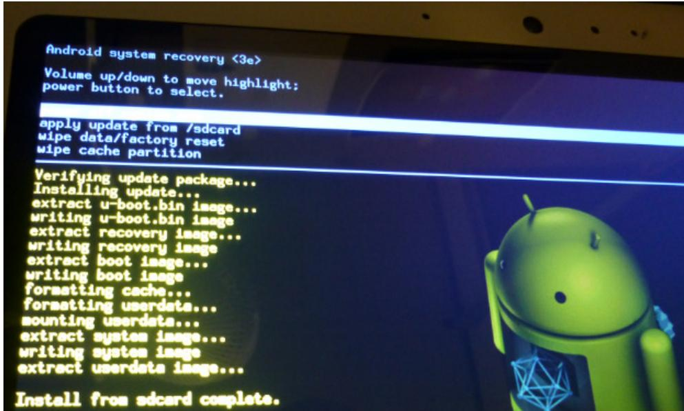
6. Hold down the Volume Down button for 10 seconds while powering up the system to go into Recovery mode
